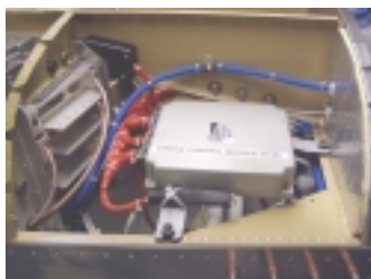
Engine Control Unit (FADEC)
