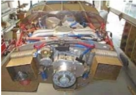
The Eggenfeller Subaru engine nestled into place
