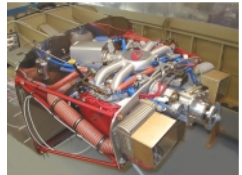
The Eggenfellner Subaru 2.5L "e-motor" in Gary Newsted's Vans RV-9A
