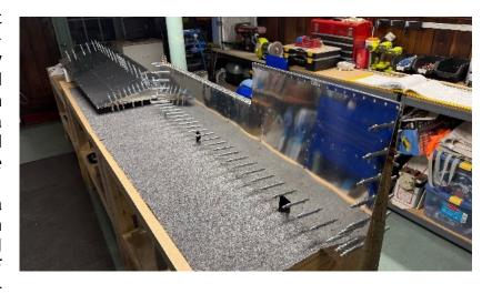
dated as my printout so there are some additional steps I spent extra time reading and trying to understand. Specifically an update that requires Proseal to help bond the elevator skins to the aft spar. It required making a 12" applicator tube and reaching that in between the already riveted in place skins, sometimes even through the holes in the forward spar after that was installed.
