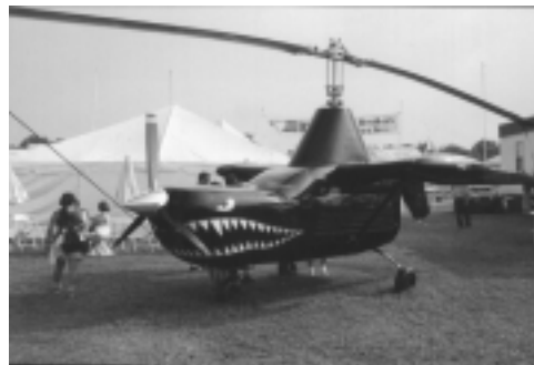
Stay outta his way! GBA's concept load-hauler made from a Cessna Skymaster airframe
