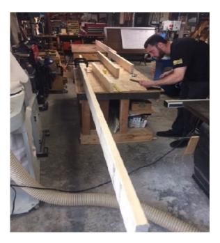
I decided to plane these edges straight so when the frame was complete, the top could be just placed on without requiring additional shimming. The method I used was to string mason line from one end to the other, on the edge to be planed. That gave me a reference on how out of straight I was. Visit my Youtube channel for a more detailed explanation of how I did this at: <a href="www.Youtube.com/">www.Youtube.com/</a>
