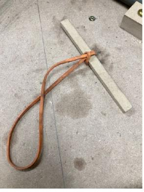
Once together, I place the tube in the approximate position in needs to be in, and wrap the rubber band around it and a supporting tube as well. I take the loop of rubber that is opposite the wood and bring the wood through it. If done properly, the wood will keep the rubber band from sailing across the room, and hold the tube in place with a bit of force.
