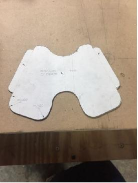
After I'm all through and the piece is finished, I just take my squeeze bottle of Acetone and soak the paper with it. In just a few minutes, the adhesive backing will soften, and with a sharp utility blade you'll be able to just easily scrape the remaining template off. A damp paper towel soaked with Acetone will get any residual glue off. Hope you found this tip useful!
